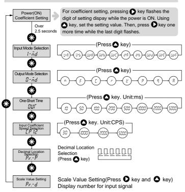
\*One-short time must be set over 50 ms. Setting under 50ms may cause malfunction.
